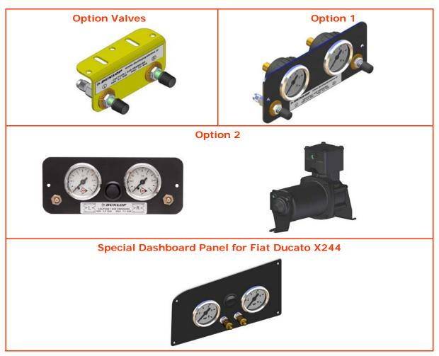
Your kit is supplied either with option valves having two valves only (above, top-left), or an optional console having both valves and pressure gauges (Option 1 or 2, or the Special Panel above). Mount the console in a position of your choice whereby it is firmly fixed, has some protection from the environment (particularly important for a console with gauges) and is easily accessible. Suggested possible locations include...
