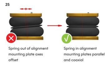
**CAUTION!** - Before fully tightening the bolts that secure the air spring to the upper and lower brackets, set the vehicle at ride height (spring height approximately 13..14 cm) and ensure that the springs are correctly aligned.
