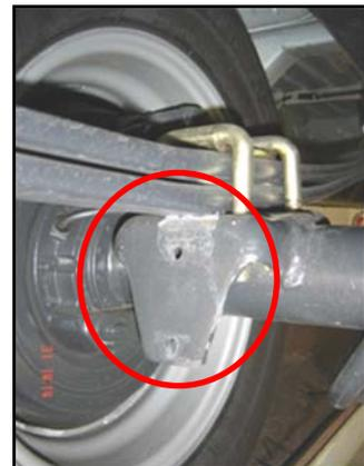
3. Reattach the stabilizer bar to the axle via the mounting brackets, at the same time attaching the lower brackets of the suspension kit. The original bolts may be used. Finger tighten only at this stage.
