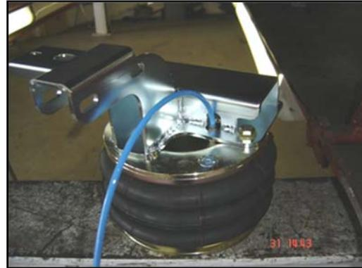
2. Attach the upper bracket to the chassis along with the bump stop. The original bump stop bolts and nuts can be used.
