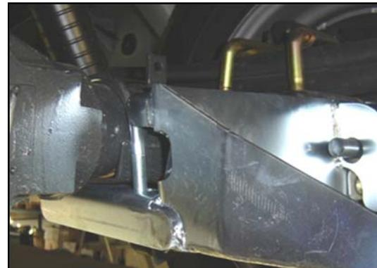
6. Tighten the nuts to the stabilizer bar bracket and the lower cross bar, so securing the lower bracket.
