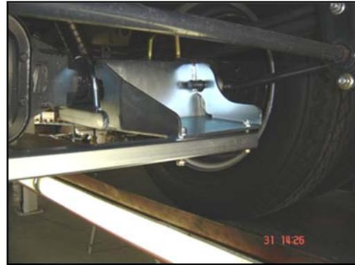
5. Temporarily remove the nuts from the M12 U-bolt that straddles the axis at each end. Pass the bolt through the holes in the lower bracket extension and then reattach the nuts in order to secure the bracket against the axle. Finger tighten only at this stage.
