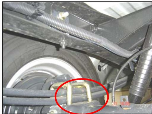
2. Remove the two bolts from the stabilizer bar mounting bracket on each side of the axle
