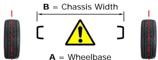
This Air Suspension Kit is suitable only when  $A - B = 565\text{mm}$
