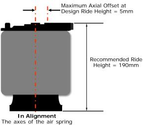
The axes of the air spring top plate and piston are parallel and coaxial.
