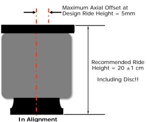
The axes of the air spring top plate and piston are parallel and coaxial.
