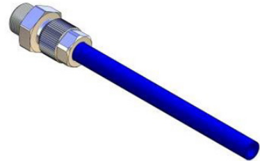
C. Feed the nut up to the connector, fully tighten by hand and finally tighten one additional turn using spanners
